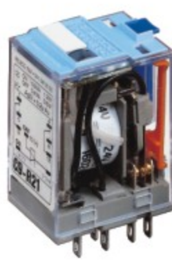
C9-R21... 磁保持继电器, 具有两对可转换触点 典型触点指标: 5A/250V AC1, 5A@30V DC1, 1A/250V AC15, 0.2A@110V DC1
