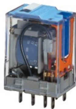
C9-E21... 灵敏型继电器, 线圈驱动功率500mW 典型触点指标: 5A/250V AC1, 3A@30V DC1
