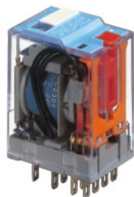
C9-A41... 通用型继电器, 具有四对可转换触点 典型触点指标: 5A/250V AC1, 5A@30V DC1, 1A/250V AC15, 0.2A@110V DC1
